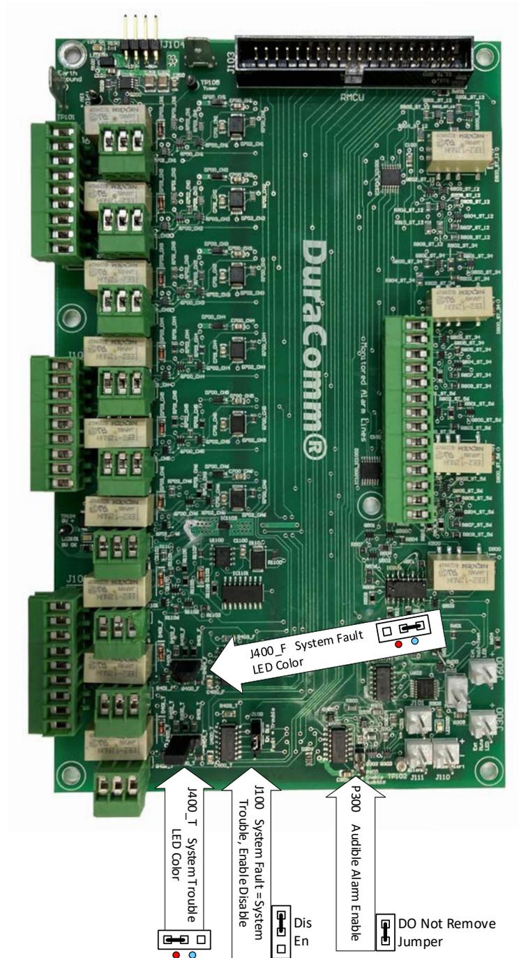
Figure 10: Annunciator Board Jumper Configuration
