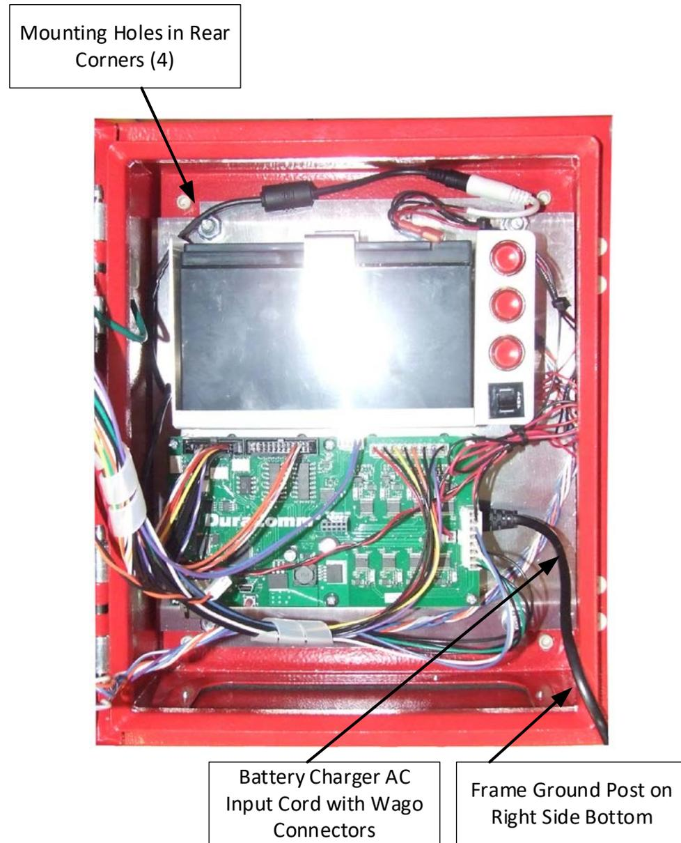
*Figure 3: Mounting Holes and AC Installation*
