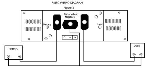
The voltage output of the charger must be at least 0.4 volts less than the voltage output of the primary system power supply. If this is not done, the charger will attempt to supply the entire system load.
