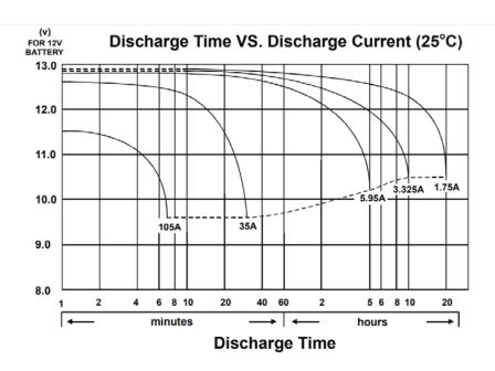
Note: This test should take about 20 hours for just the discharge cycle with a 2 Amp load and a new 35 Amp-Hour battery.
