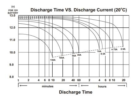
Note: This test should take about 24 hours for just the discharge cycle with a 2 Amp load and new 50 Amp-Hour batteries.
