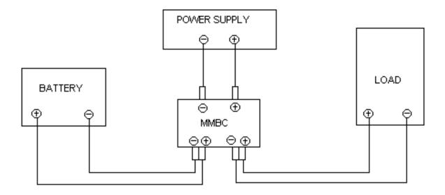
Wire according to the diagram, carefully observing polarity, and using wire large enough for the amperage capacity of your system. MMBC input and output terminals will accept parallel #10 AWG, or up to single #4 AWG. (See wire chart on page 3 for guidelines)
