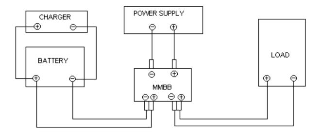
Wire according to the diagram, carefully observing polarity, and using wire large enough for the amperage capacity of your system. MMBB input and output terminals will accept parallel #10 AWG, or up to single #4 AWG. (See wire chart on page 3 for guidelines.)
