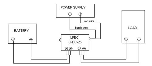
Wire according to the diagram, carefully observing polarity, and using wire large enough for the amperage capacity of your system.
