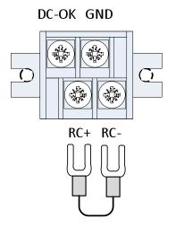
(Shown with factory jumper for PSU ON)
