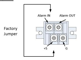
(Shown with factory jumper to silence alarm condition)
