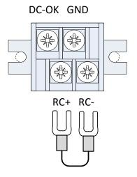
(Shown with factory jumper for PSU ON)
