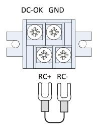
(Shown with factory jumper for PSU ON)
